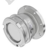
Coupling should be according to EN14420 and it shall be manufactured by forging and also it should be engraved ISO/EI standard, serial no. , date of manufacture & name of manufacture. Operating temperature  $5^{\circ}$  C to  $50^{\circ}$  C.
